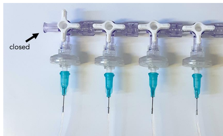
Figure 13 – Assembly of the ramp. Pay attention to set the valves as displayed in figure, so that air can pass through each needle.
